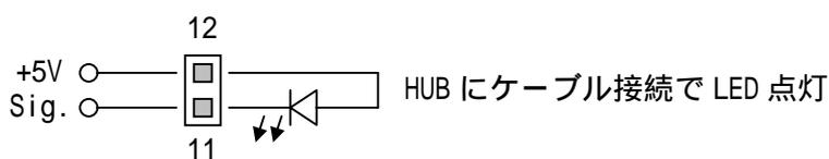
D : Ethernet CRS (Carrier Sense) LED
